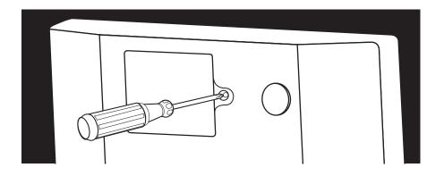
Insert 3 x 1.5V "AA" or R6 size batteries. Alkaline batteries recommended. Replace cover and tighten screws.
