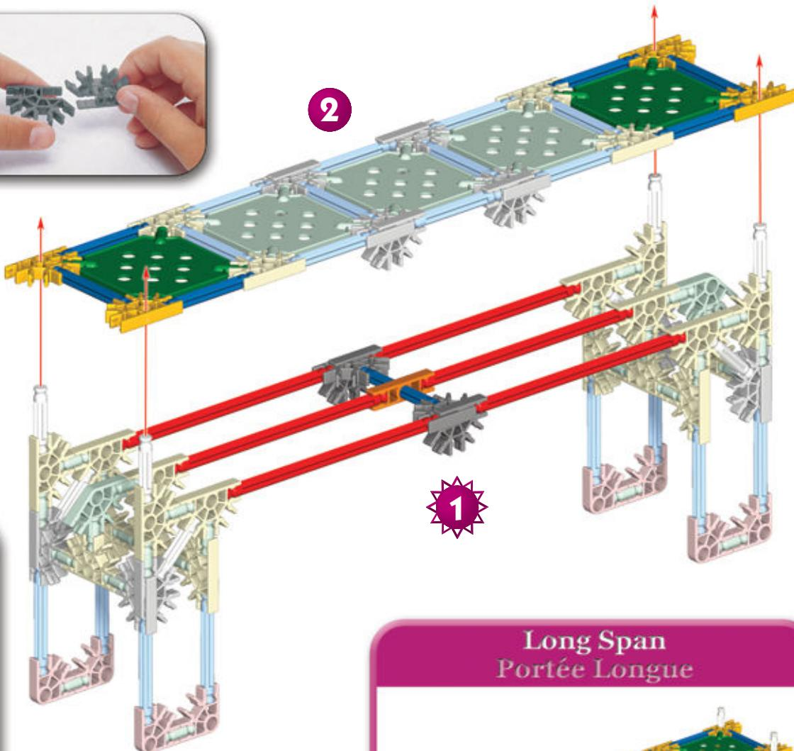
The beam bridge is the most basic bridge type. It is made of a horizontal beam resting on piers at each end, like a wooden plank lying across two logs.
