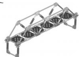
Fig. 27 King Post truss design
