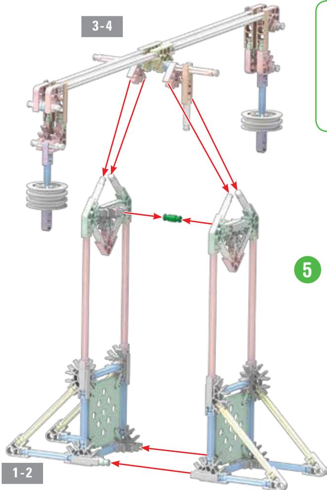
A balance is a 1st class lever. It weighs things like letters and apples. To make a balance work, you put the thing to weigh (the resistance) on one side, and weights (the effort) on the other. The fulcrum is in the middle. When the objects equal the same amount, the balance arm will be perfectly straight (level). If you move the resistance close to the fulcrum, you need less effort to balance it.
