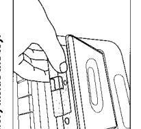
1. Pull open the cassette compartment door by the corner tab. 2. Insert the cassette with the tape side you would like to play facing forwards.
