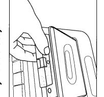
1. Pull open the cassette compartment door by the corner tab. 2. Insert the cassette with the tape side you would like to play facing forwards.
