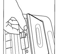
Pull open the cassette compartment door by the corner tab. 2. Insert the cassette with the tape side you would like to play facing forwards.
