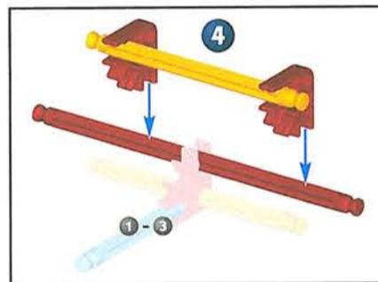
It's very important to position blue and purple Connectors in a specific direction. Pay close attention to the instructions, and position these Connectors horizontally or vertically exactly as they are shown. Push together tightly until you hear a "click".
